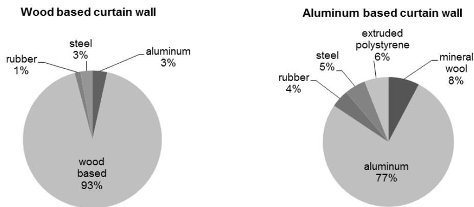
**Figure 4: Mass distribution of the materials in the wood-based and aluminum curtain wall (an opaque variant) with the dimensions of 3.3 (h) x 1.5 (w) meters.**
