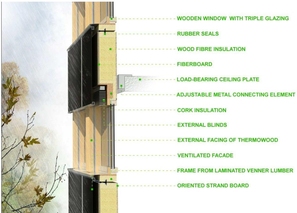
Figure 2: Scheme of a curtain wall made of wood-based panels.
